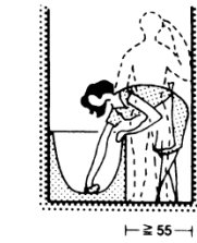
⑫ Minimum space between bath and wall
